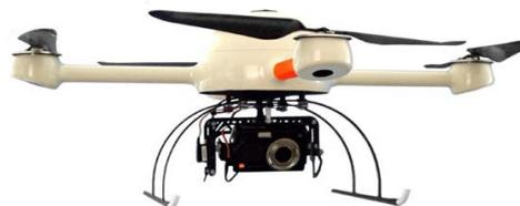
Figure 1: Micro-drone md4-200 with attached PENTAX Optio A40.
