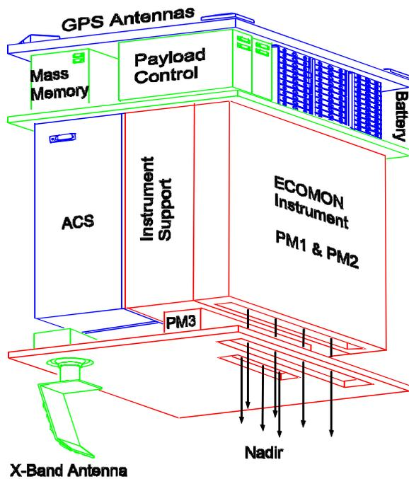
Figure 5: S/C's instrument accommodation
