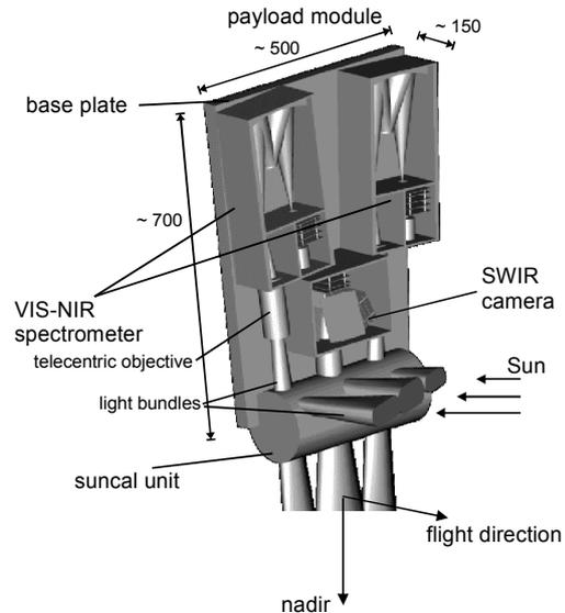
Figure 3: Mounting scheme of the payload module (PM)
