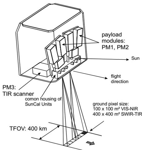
Figure 2: ECOMON S/C with three payload modules
