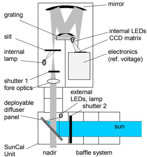
Figure 4: In-flight calibration tools for the imaging spectrometer
