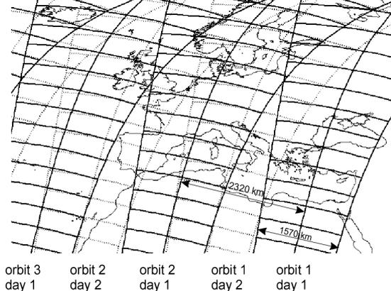
Figure 1: Descending passes for Sun-synchronous orbits
