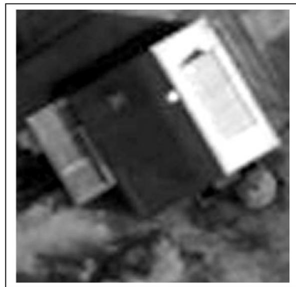
Figure 7: Results of the mosaiking process: The center of the virtual DMC image is located in the center of the dark roof. The tie point extraction, the lens distortion correction and the rectification has been done. The four edges of the panchromatic images fit perfectly together as shown in the left image. After applying a blending algorithm, even the radiometric differences between the images are removed (right image).
