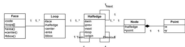
Figure 1: UML Diagram of the extended DCEL
