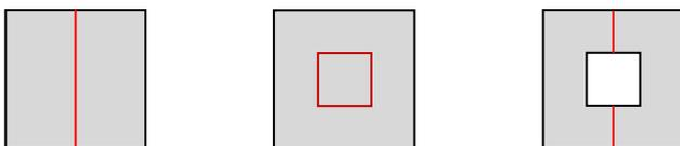
Figure 3: Beside the obvious cases (left and middle) of a merge, where the number of loops is reduced there are also cases which produce new inner loops (right).
