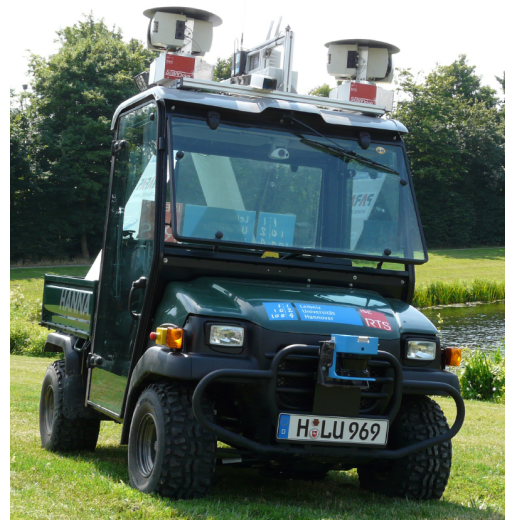
Figure 1: The RTS Hanna robotic vehicle. The point clouds were acquired using the four laser scanners mounted on the two ScanDrives on top of the vehicle. Image courtesy of RTS.
