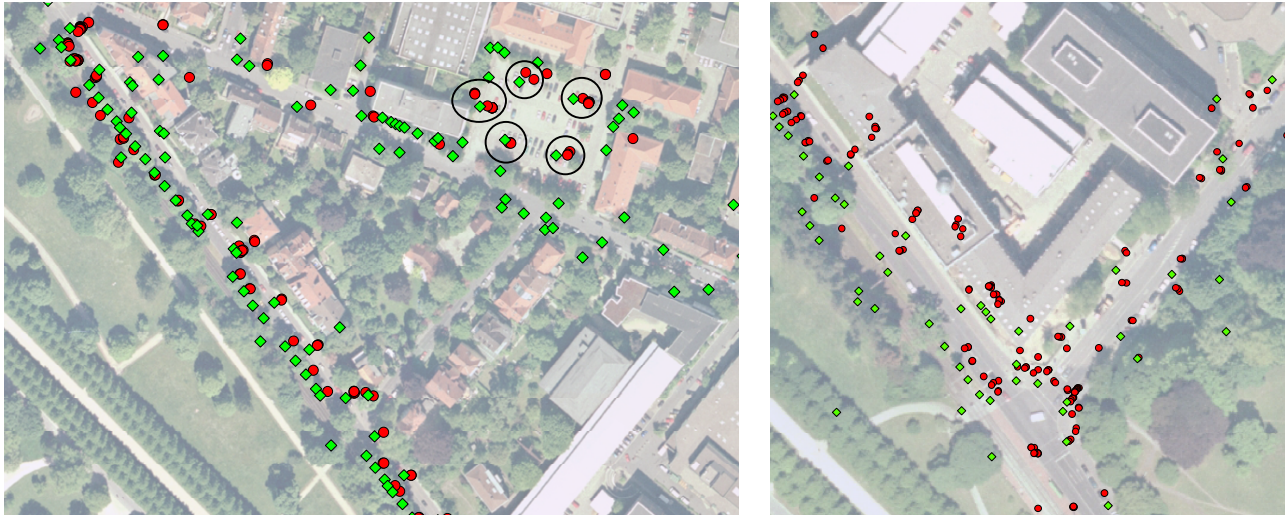
Figure 7: Comparison of reference poles (green squares) and poles extracted using the RTS Hanna vehicle (red dots).
