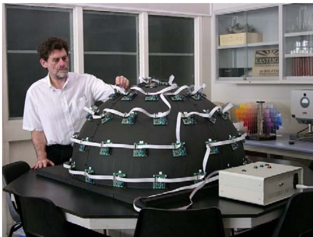
Figure 2. Hemispherical acrylic dome with 64 flash lamps.
