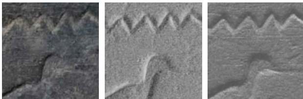
Figure 6. (left) Detail of 150x150 pixels of an image from lamp 34 (Tier 3). Normals were computed from the green channel for three-lamp combination 17-36-58: (centre) X normal; (right) Y.
