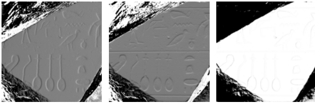
Figure 5. Images of normals in the X,Y and Z directions extracted from the PTM representation.
