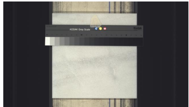
Figure 2. Sample image 2098x1200 pixels, with marble tile and Kodak Q-13 Gray Scale reference card
