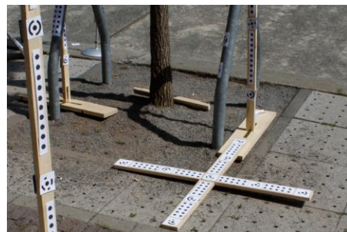
Figure 1: Detail view of markers (encoded and unencoded) placed around a tree
