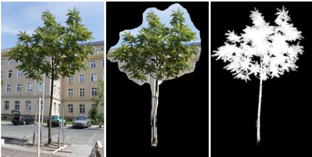
Figure 2: Alpha matting of an image using the closed form matting algorithm by (Levin et. al 2008). Left: the original image; Middle: image with scribbles by user-input; Right: resulting alpha image, separating the image in fore- and background.
