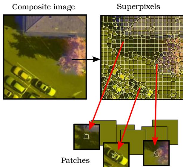
Figure 1: Patch generation from composite image
