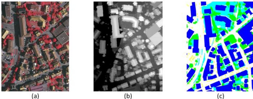
Example patches of the semantic object classification contest with (a) true orthophoto, (b) DSM, and (c) ground truth
