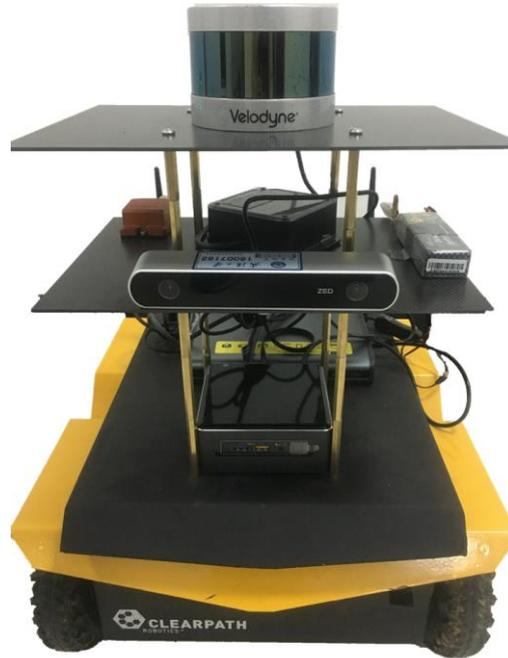
Fig. 4 UGV 3D mapping system.
