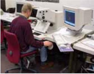
Manual measurements on analogue stereo images with an analytical plotter
