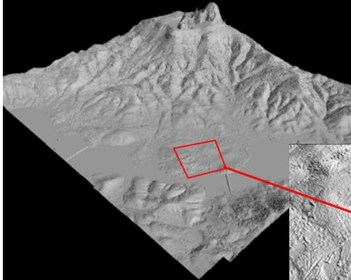
3D Visualization of 5 m Grid DSM
